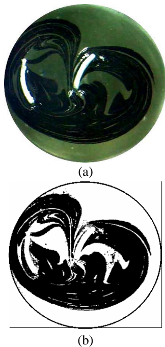
Fig. 4. Typical photo of (a) the actual one and (b) the processed one ( L = \frac{\pi}{3} R_b , \omega_{ave} = 15 ( Re \approx 10 ), t=36s ).
