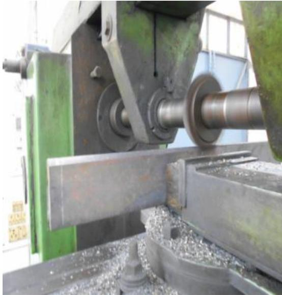
Fig. 3. V-groove making on milling m/c.
