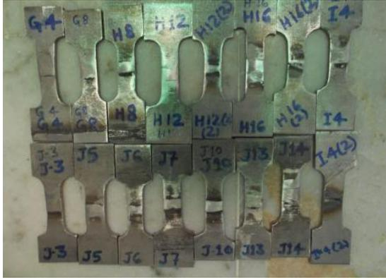
Fig. 7. Actual tensile test specimens.
