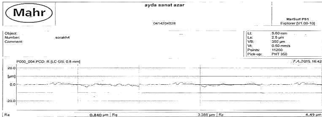
Fig. 9. Surface roughness profile of the first hole (drilled with 0.06 (mm/rev) feed rate, 500 (rpm) spindle rotation speed, and cutting fluid containing 90 \mu\text{m} alumina particles).
