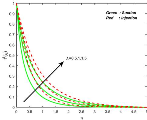
Fig. 8. Velocity field for different values of material parameter.
