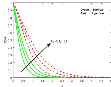
**Fig. 15.** Temperature field for different values of nonlinear thermal radiation.
