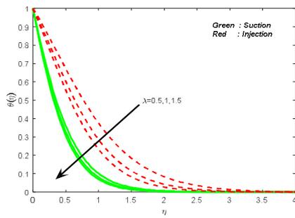
**Fig. 18.** Temperature field for different values of stretching ratio parameter.
