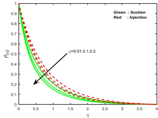
**Fig. 5.** Velocity field for different values of ferroparticle volume fraction.
