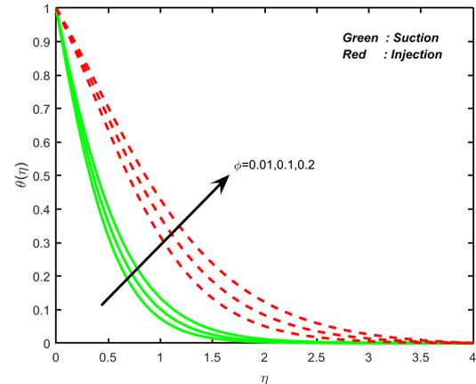
**Fig. 7.** Temperature field for different values of ferroparticle volume fraction.
