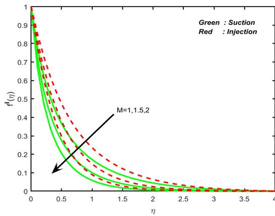
**Fig. 2.** Velocity field for different values of magnetic field parameter.
