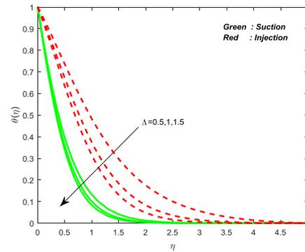
Fig. 10. Temperature field for different values of material parameter.
