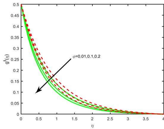
**Fig. 6.** Velocity field for different values of ferroparticle volume fraction.
