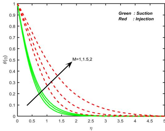
**Fig. 4.** Temperature field for different values of magnetic field parameter.
