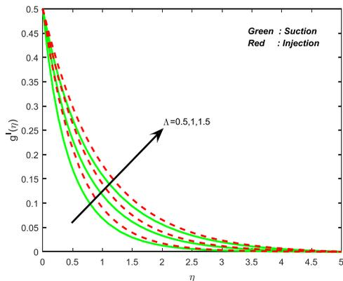
Fig. 9. Velocity field for different values of material parameter.
