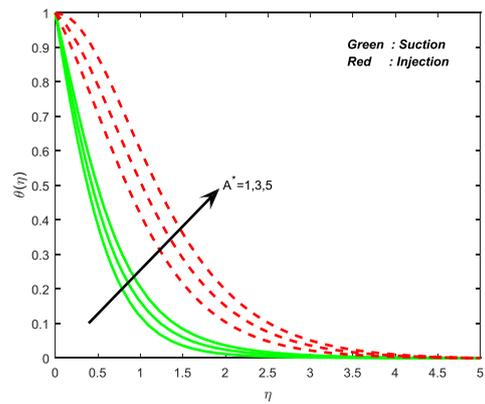
**Fig. 14.** Temperature field for different values of non-uniform heat source/sink.
