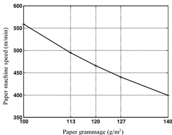
Fig. 6. Paper machine speed variation vs. paper grammage.
