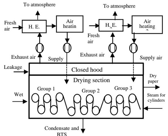
Fig. 1. The studied drying section and its heat recovery system.
