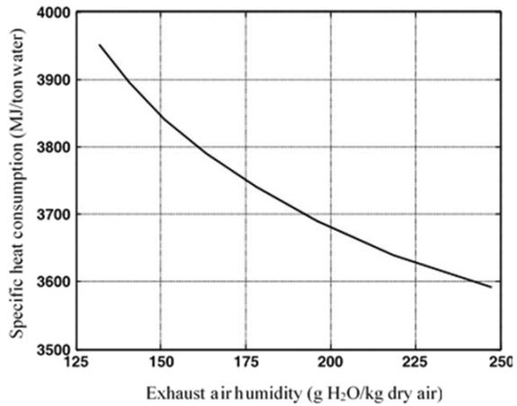
Fig. 14. SHC<sub>water</sub> at various exhaust humidity.
