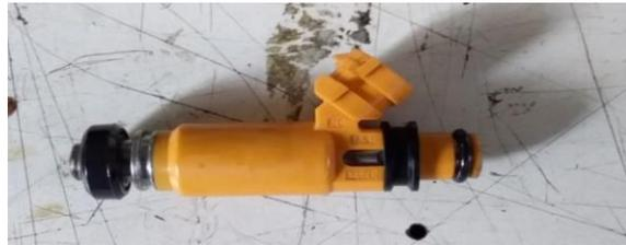
Fig. 5. Port fuel injector.
