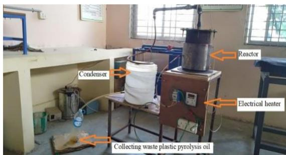
Fig. 2. Pyrolysis equipment.
