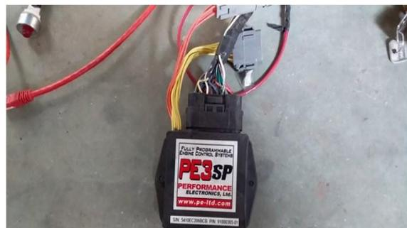
Fig. 7. Photo graphical view of ECU.
