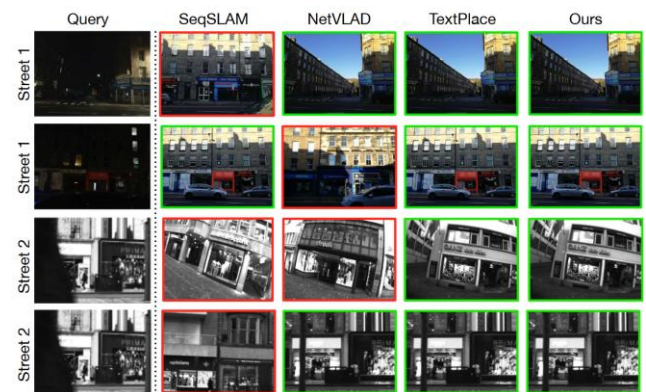
Fig. 4: Qualitative comparison of the proposed model with SOTA methods [2], [22], [45] on the SCTP dataset. The correct and incorrect results are bounded with green and red colors.
