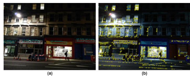
Fig. 1: Comparing the (a) Text features used in the proposed E2E text detection model and (b) Key point features used in different VPR techniques [11], [45]. Text features are shown with 'cyan' color boxes, and the 'x' marks with 'yellow' color denote the keypoint features.
