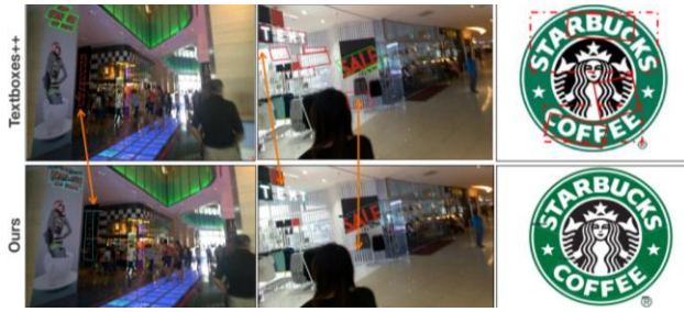
Fig. 6: Comparison between the proposed end-to-end model (bottom row) with Textboxes++ [34] algorithm (top row). The red boxes in the top row images show the failure cases (Images are taken from [34]), and the cyan text and boxes show our results. The orange arrows point to text regions where the proposed model could successfully predict failure text instances of Textboxes++.
