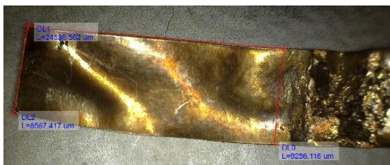
Fig. 9. Final fabricated IPMC.
