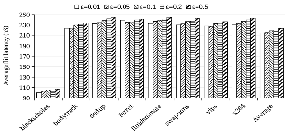
Fig. 8: The effect of \epsilon on the average flit latency of the NoC.
