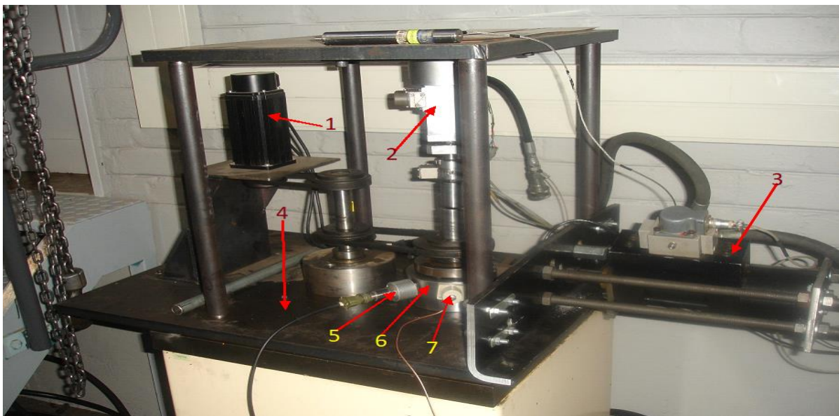
1.Variable speed motor, 2.Axial hydraulic actuator, 3.Radial hydraulic actuator, 4.Test rig, 5.Acoustic transducer 1, 6.Test bearing housing, and 7.Acoustic transducer 2
