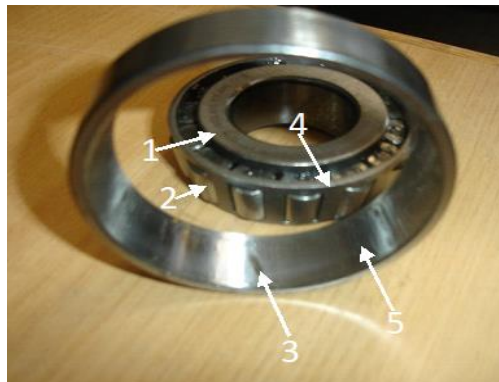
1. Bearing inner ring, 2. Bearing roller, 3. Seeded crack, 4. Rollers cage, and 5-Bearing outer ring
