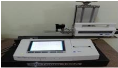
Fig. 4. Surface roughness measuring instrument (Surfcom 130A).
