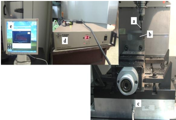
Fig. 8. CF measurement; (a) tool, (b) workpiece, (c) dynamometer, (d) processing system, and (e) software.
