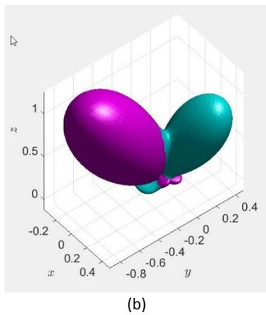
Fig. 3:  $|y(\theta, \phi)|$  for MPDR beamformer. (a) contour plot, arrival direction of the disturbance plane wave and desired plane wave are indicated by the white "+". (b) balloon plot.
