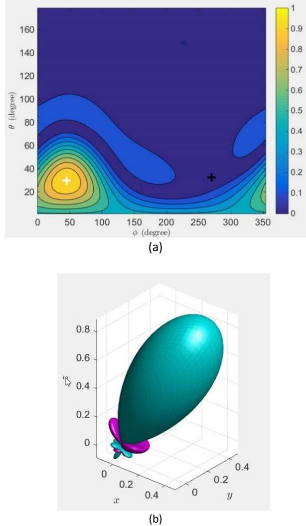
Fig. 2:  $|y(\theta, \phi)|$  for MVDR beamformer with the cross-spectrum matrix of noise obtained by the proposed method. (a) contour plot, arrival direction of the desired plane wave is indicated by the white “+” and the arrival direction of the disturbance plane wave is indicated by the black “+”. (b) balloon plot. In this plot cyan color represents positive values of  $\text{Re}\{y(\theta, \phi)\}$ , and magenta color represents negative values of  $\text{Re}\{y(\theta, \phi)\}$ .
