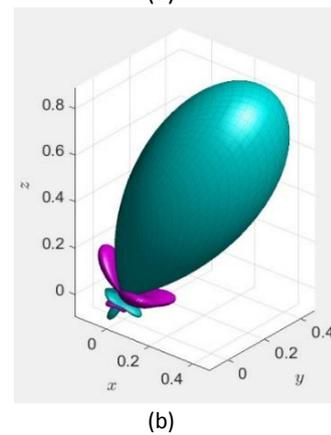
Fig. 5:  $|y(\theta, \phi)|$  for MVDR beamformer which use the cross-spectrum matrix of noise obtained by the proposed method. (a) contour plot, arrival direction of the disturbance plane wave is indicated by the black "+", and the arrival direction of the desired plane wave is indicated by the white "+". (b) balloon plot.
