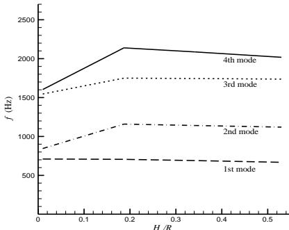
**Fig. 13.** Effects of torispherical head depth on the natural frequencies (Hz) of the structure with clamped-free boundary condition.
