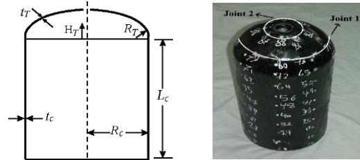
**Fig. 1.** Test sample and geometry.
