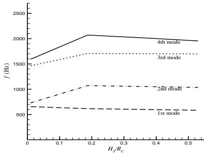
**Fig. 12.** Effects of torispherical head depth on the natural frequencies (Hz) of the structure with simply supported-free boundary condition.
