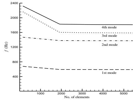
**Fig. 2.** Effect of number of elements on the natural frequency (Hz).
