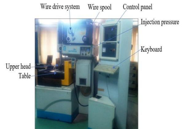
Fig. 1. Sprint cut CNC WEDM machine tool.
