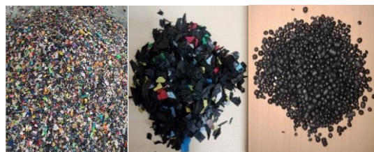
Fig. 2. Pelletized recycled high impact polystyrene from disposable cups.
