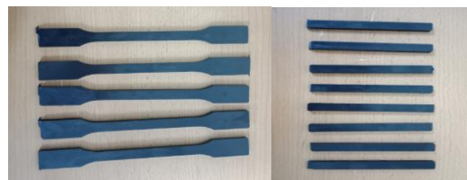
Fig. 3. Tests specimens according to ISO 294-1 and ISO 294-2.
