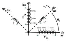
Fig. 2: The schematic of the resolver's windings.
