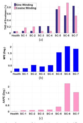
Fig. 7: The performance of the studied resolver under different fault conditions: (a) THD of envelopes, (b) MPE, and (c) AAPE.
