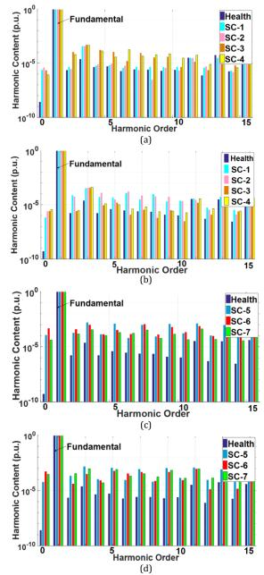
Fig. 6: The harmonic content of the voltages' envelope: (a) for the sine voltage (independent faults), (b) for the cosine voltage (independent faults), (c) for the sine voltage (simultaneous faults), and (d) for the cosine voltage (simultaneous faults).
