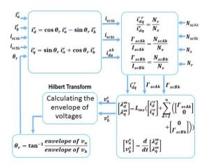
Figure 4: The block-diagram of the simulation.
