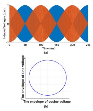
Fig. 5: The results of the healthy sensor obtained from the proposed model: (a) Analogue voltages, (b) The envelope of sine voltage versus that of cosine voltage.
