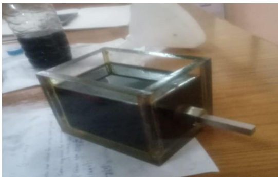
Fig. 6. Oil chamber for breakdown voltage measurement with sample oil.
