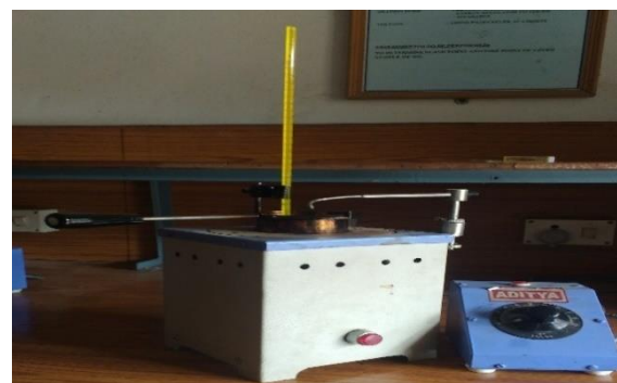
Fig. 8. Cleaveland flash & fire point apparatus during conducting of experimentation.
