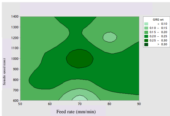
Fig. 8. Contour plot of GRG Vs spindle speed and feed rate.
