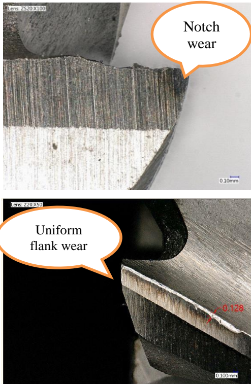
Fig. 12. Notch wear and uniform flank wear ( v=18 m/min, nanofluid with emulsion 5%)
