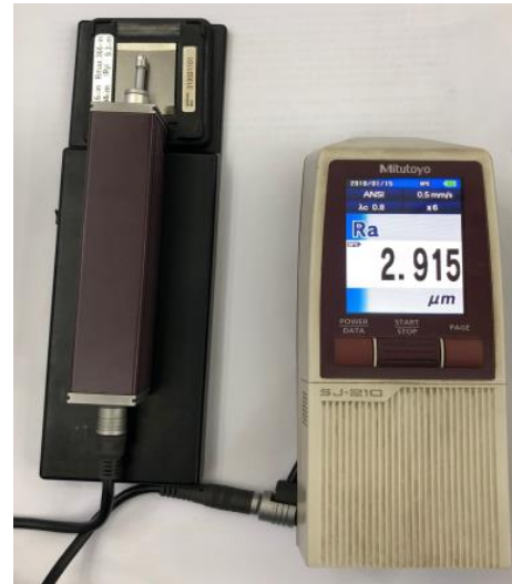
Fig. 1. The portable surface profilometer Mitutoyo SJ-210 used for the roughness measurement.
