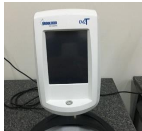
Fig. 2. DV2T™ viscometer for measuring the viscosity of nanofluids.
