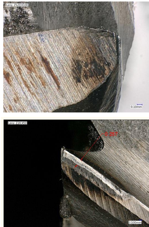
Fig. 14. Notch wear and uniform flank wear ( v=30 m/min, nanofluid with emulsion 5%) at 40 minutes
