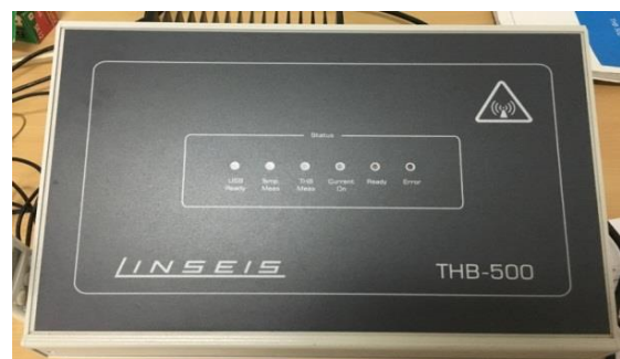
Fig. 3. Linseis THB 500 for measuring the thermal conductivity of nanofluids.
