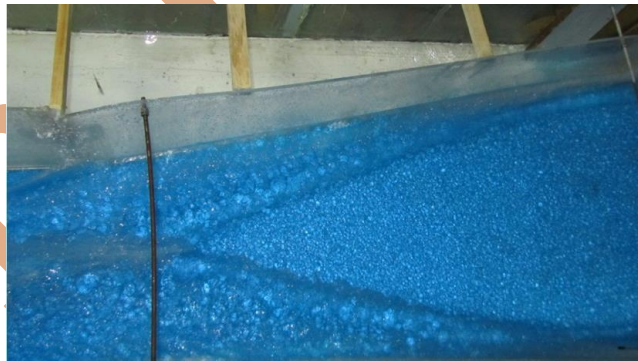
Fig. 2. Formation of the shock waves in the model 1 for Fr_1=7.0
