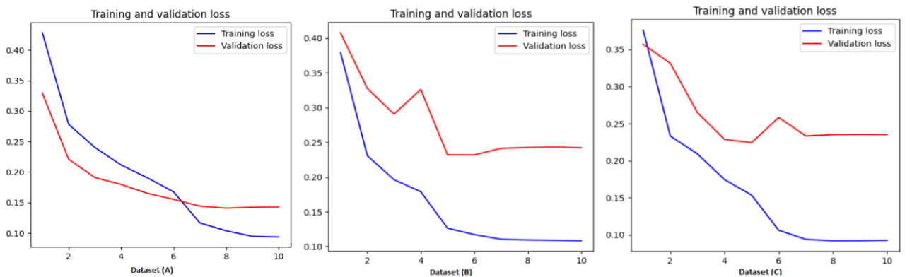
Fig. 9: Learning and validation curves for CBiLSTM on datasets A, B, and C where the minimum loss values are 0.147 (Epoch 8), 0.232 (Epoch 5), and 0.226 (Epoch 5).
