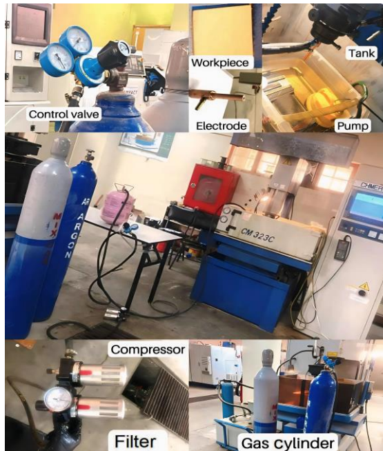
Fig. 1. The developed experimental facility for the wet, near-dry, and NDPM-EDM processes.
