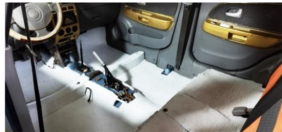
Fig. 9. Replacement of carpet mat with nano polyester insulation.
