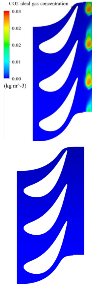
Fig. 18. Distribution of CO 2 concentration in a plane close to the hub: (a) \Phi_0 = 0.21 and (b) \Phi_0 = 0.003 .
