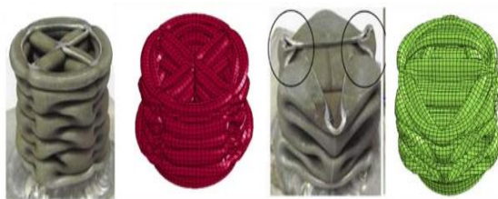
Fig. 2. Deformation mode of double and quadruple experimental cell structure [6] and present simulation.
