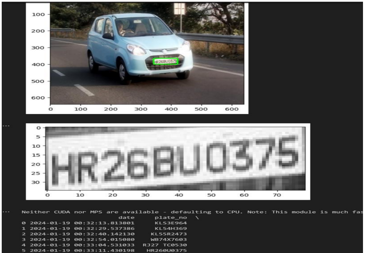
Fig. 16: Image processing of vehicle with plate number HR26U0375: plate number detection, segmentation and capturing with time stamps.
