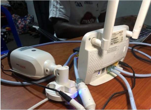
Fig. 4: Rare view of the IP camera set-up with an RJ-45 cable and a router.
