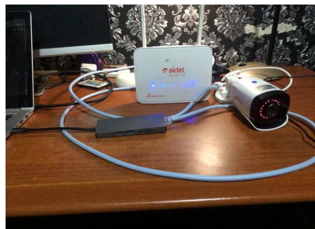
Fig. 3: Front view of the IP camera set-up with an RJ-45 cable and a router.
