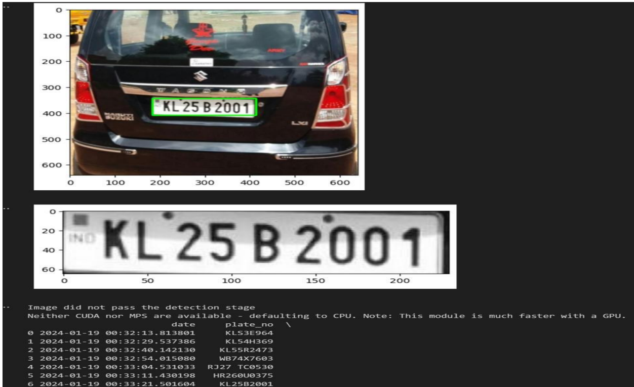
Fig. 17: Image processing of vehicle with plate number KL 25B 2001: plate number detection, segmentation and capturing with time stamps.
