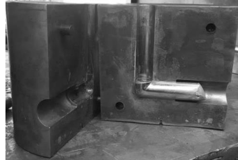
Fig. 2. ECAP-die and manufactured ECAPed copper.
